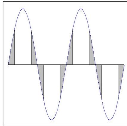
The mechanical switching mechanism of the RCD uses energy from the mains to trip. The shaded areas of the waveform above, indicate dead spots where a signal to trip the RCD will be ignored until there is sufficient energy in the next half cycle.
