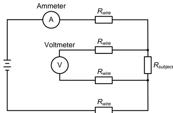
$$R_{subject} = \frac{\text{Voltmeter indication}}{\text{Ammeter indication}}$$
