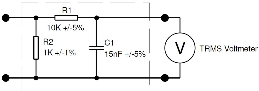
***Touching the protectively earthed case of a Class I device and opening up the earth return line via the lead will mean that the TOUCH CURRENT IS EARTH LEAKAGE CURRENT. Touching the protectively earthed case with the earth line intact is a waste of time as the current will always be close to zero as you have the 1K $\Omega$  MD in parallel with a maximum of 0.3 $\Omega$ .***
